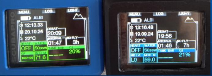
compensate for the different calculation with the GF 100/100 of the G2 TEK with the MB Level = L0 of the G2 (Thus the difference in "MOD" ...). But anyway the G2 TEK had longer "NDL" and went always quicker into NDL = 99 and had shorter "NO FLY" than the G2 ...
